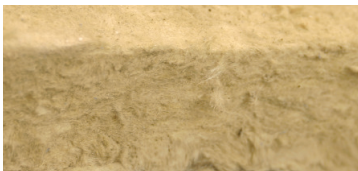
mineral wool (reduces heat loss & acoustics)
